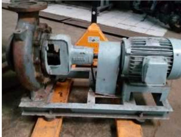
Gambar 3.1 Pompa Sentrifugal Merk Ebara
