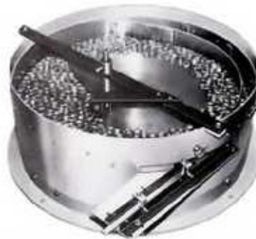
Gambar 2.2 *rotary feeder*
