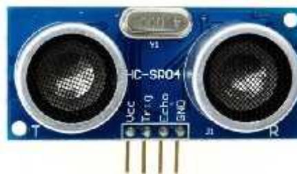
Gambar 2.11 Sensor Ultrasonik
