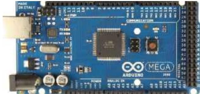
Gambar 2.4 Arduino Mega 2560
