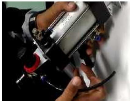
Gambar 3.3. Pemasangan selang regulator – *handle*
