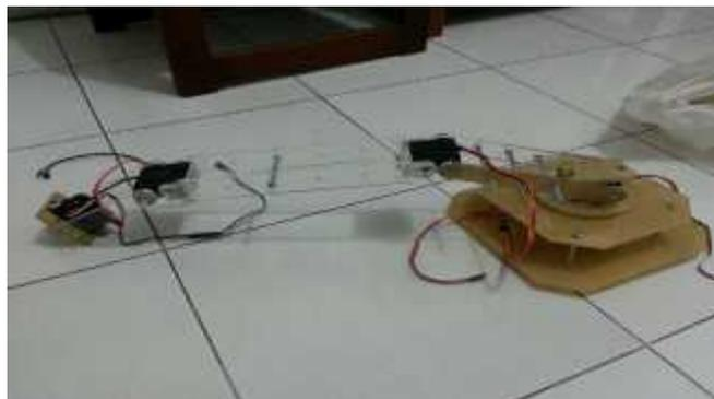
**Gambar 3.8 Hasil Rancang Bangun Arm Robot Tanpa Gripper**
