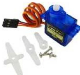
Gambar 2.9 Motor Servo SG-90
